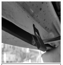
4. With both holes drilled out use a flat head screwdriver to pry on plastic trim and slide in the U-nuts.
