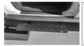
6. Re-install your step and with the 3/16" Allen wrench and 1/2" socket fully tighten all four button head screws.
