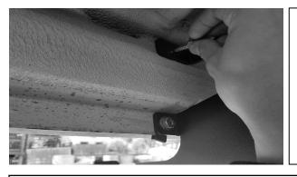
7. Fully tighten both 5/16" bolts to U-nuts. Finally with a 3/8" socket install the #14 selftapping screws to both brackets and be careful not to over tighten them. Your step is now fully installed.
