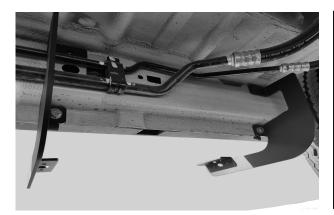
5. With both Unuts in place use the 5/16" bolts and washers to secure both brackets to the rocker panel. Do not fully tighten.
