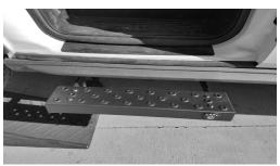
6. Re-install your step and with the 3/16" Allen wrench and 1/2" socket fully tighten all four button head screws.
