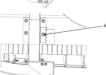
.6. A very important step in the installation process, make sure to tighten this nylon lock nut so the bolt only comes through an 1/8". If this nylon lock nut gets over-tightened, it will be very difficult to install the front bolts later in step 10.
