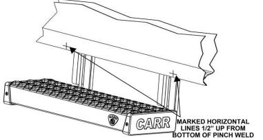
Transfer the marks from the previous step and mark the front and rear step on the outside body metal as indicated on this drawing. Center punch marked lines. With the variable drill motor, using plenty of cutting oil, take a 3/16" **solid carbide** drill bit and drill out at a slow speed the centered punched holes. Again, using plenty of cutting oil and at a slow speed, drill out the 3/16" hole with the 5/16" **solid carbide** drill bit.
