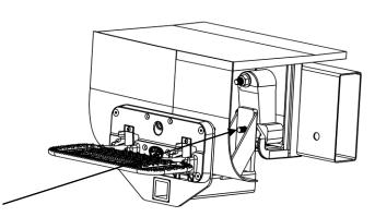
With the step assembly on the bolt, screw the nut back on to the vehicle only half way. DO NOT— TIGHTEN.
