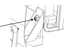
4. From underneath the step assembly, line up the slot in the tab of the step assembly with the slot on the bottom of the spring shackle assembly on the vehicle.
