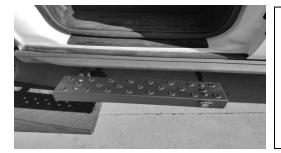
6. Re-install your step and with the 3/16" Allen wrench and  $\frac{1}{2}$ " socket fully tighten all four button head screws.
