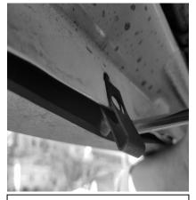
4. With both holes drilled out use a flat head screwdriver to pry on plastic trim and slide in the U-nuts.
