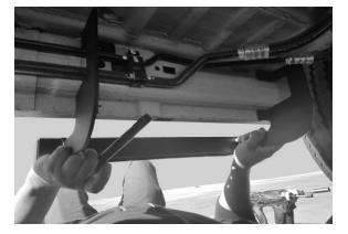
2. With step assembled, place step in the desired location avoiding any A/C lines as shown (Passenger vans only) Avoid any bumps or indents to allow both brackets to be parallel to each other. With a marker mark both holes for the 5/16" mounting hardware; top holes do not need to be marked. **NOTE: Passenger van with A/C lines shown.**
