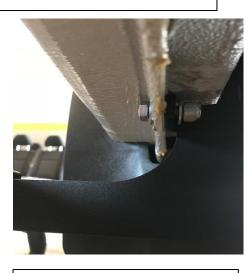
4. With step disassembled and both holes drilled, Use the 5/16 hex bolts to mount brackets as shown. Do not fully tighten.
