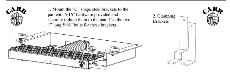
3. Place the clamping brackets alongside the frame using the 1/2" hardware provided and hand tighten. Make sure the clamp assembly is up against the rubber muffler assembly. This alignment is critical for the step to be in its proper location.
