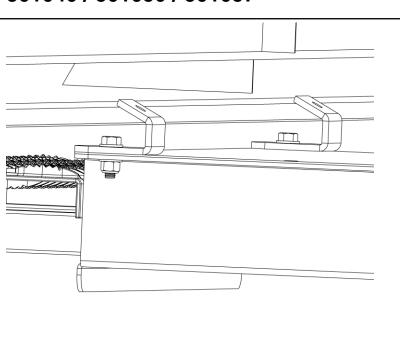
6. Take the two 1" long 5/16" bolts with washers and nylon lock nuts and securely tighten the "C" shaped steel brackets to the vehicle's rocker panel.
