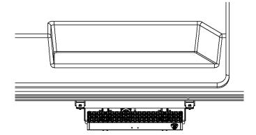
2. From underneath vehicle, position the step assembly centered on the open step area of the van as shown. You will need to use a floor jack or some way to hold the step in this position for the next step.
