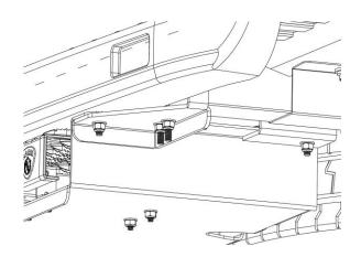
12. Once all the hardware has been installed, securely tighten the step assembly to your vehicle. Push on the step to deploy it. Then push it in to lock it in place.
