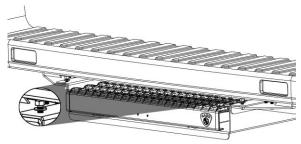
11. Take two 5/16" hex bolts with washers and insert them in the front holes of the Main Brackets so they go through the pan. The first bolt and washer will be fairly easy to install. The second one may be more difficult. Wiggle the entire assembly if the fit is tight until the bolt and washer are installed. Take two washers and two nylon lock nuts and hand-tighten to these bolts.
