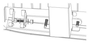
4. Take one of the hex head bolts with two washers and a nylon lock nut and hand-tighten this hardware to the vehicle and the Long "L" Bracket shown in the diagram.
