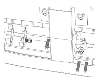
5. Take one of the "C" Brackets and slide it on to the shorter carriage bolt with a washer and nylon lock nut and only hand-tighten. Place two additional longer carriage bolts through the two holes at the bottom of the "C" Bracket. See diagram.
