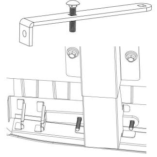
2. Take one of the Long "L" Brackets and insert one of the longer carriage bolts as shown.
