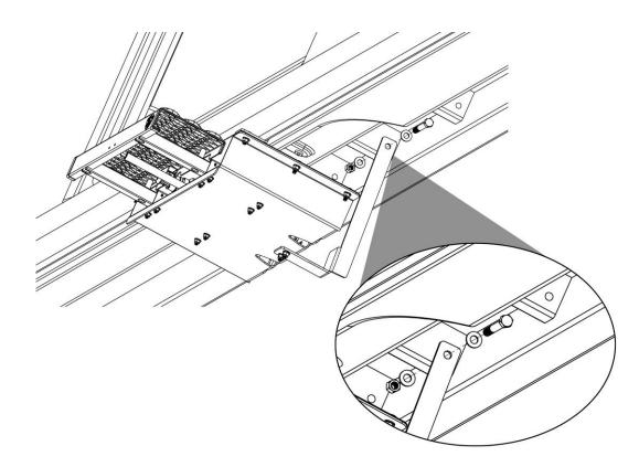
3. Take the entire step assembly and lift it up inside the vehicle behind the side door. It is highly recommended to use a floor jack or something to rest the step assembly on while completing this step. Make sure the Rear Steel Bracket is up against the middle cross member as shown. Take the <sup>1</sup>/<sub>2</sub>" hardware and assemble it to the vehicle but only hand tighten. This 1/2" bolt assembly will be tightened in step 7.
