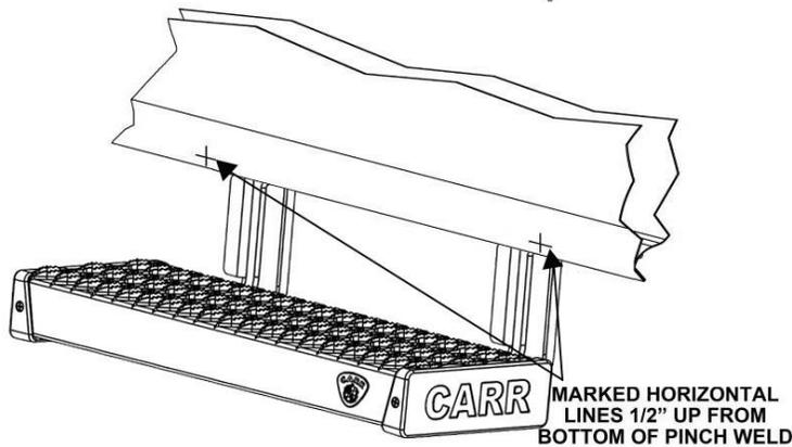
Transfer the marks from the previous step and mark the front and rear step on the outside body metal as indicated on this drawing. Center punch marked lines. With the variable drill motor, using plenty of cutting oil, take a 3/16" **solid carbide** drill bit and drill out at a slow speed the centered punched holes. Again, using plenty of cutting oil and at a slow speed, drill out the 3/16" hole with the 5/16" **solid carbide** drill bit.
