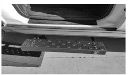
6. Re-install your step and with the 3/16" Allen wrench and 1/2" socket fully tighten all four button head screws.
