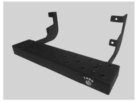
1. Assemble step as shown by using a left and a right bracket with tabs facing inwards. Use 5/16" x1" socket button head screws with washers and nylon locks nuts. Securely tighten step Do not fully tighten.
