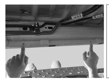
3. With both holes marked, center punch both marks and drill out with the 1/8" drill bit followed by the 5/16" drill bit. Try to clean out burs as best as possible. Be careful not to drill into plastic trim. The step and brackets will need to be disassembled for the next step.
