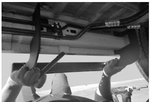
2. With step assembled, place step in the desired location avoiding any A/C lines as shown (Passenger vans only) Avoid any bumps or indents to allow both brackets to be parallel to each other. With a marker mark both holes for the 5/16" mounting hardware; top holes do not need to be marked.
