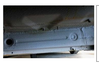
3. With both holes marked, center punch both marks and drill out with the 1/8" drill bit followed by the 5/16" drill bit. Try to clean out burs as best as possible. The step and brackets will need to be disassembled for the next step.
