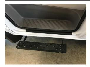
6. Re-install your step and with the 3/16" Allen wrench and 1/2" socket fully tighten all four button head screws.
